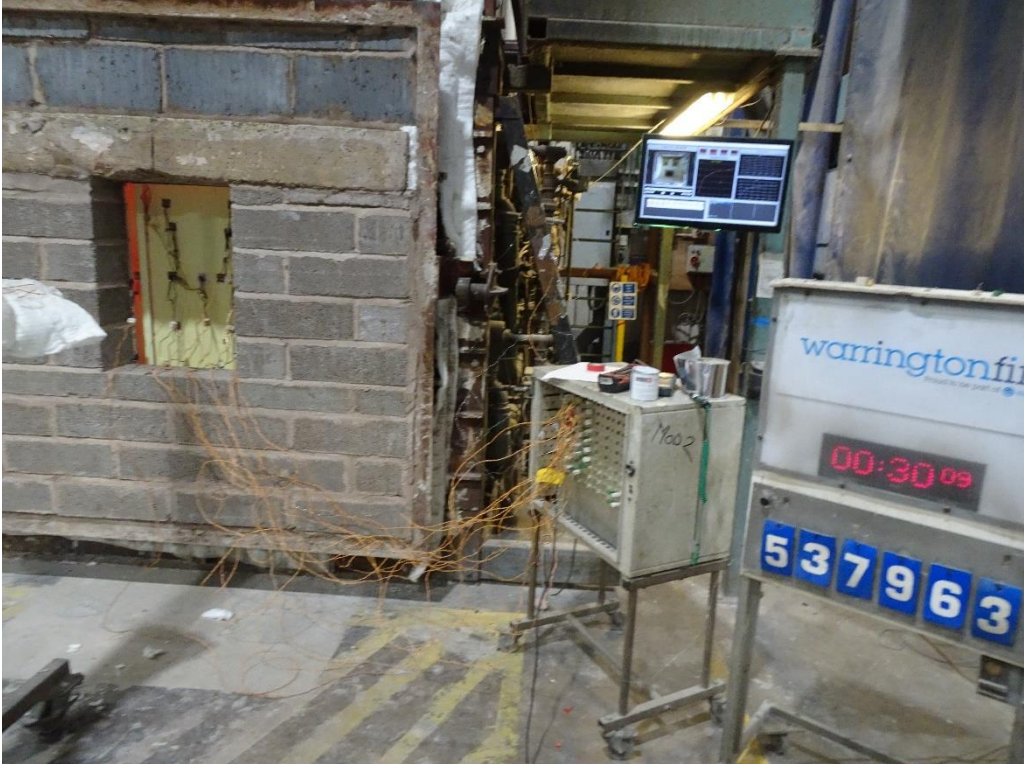
The unexposed face of the electrical box after a test duration of 30 minutes
