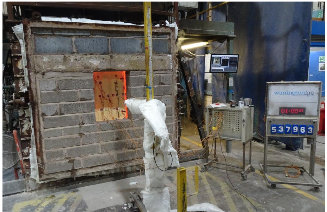
The unexposed face of the electrical box after a test duration of 60 minutes
