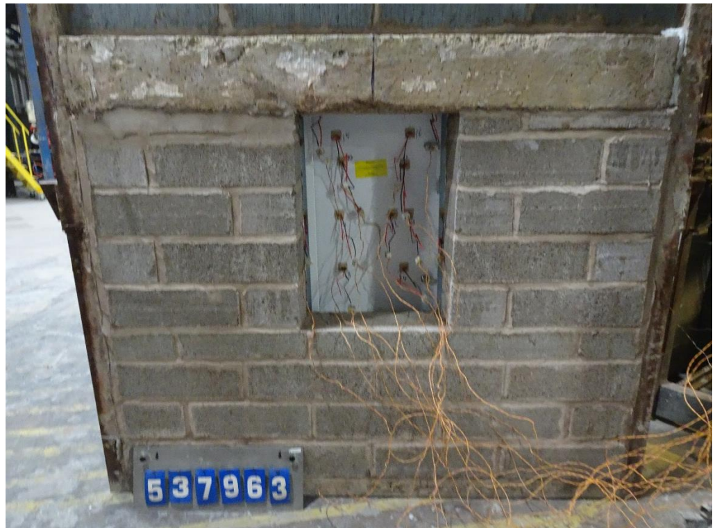
The unexposed face of the electrical box prior to the start of the test
